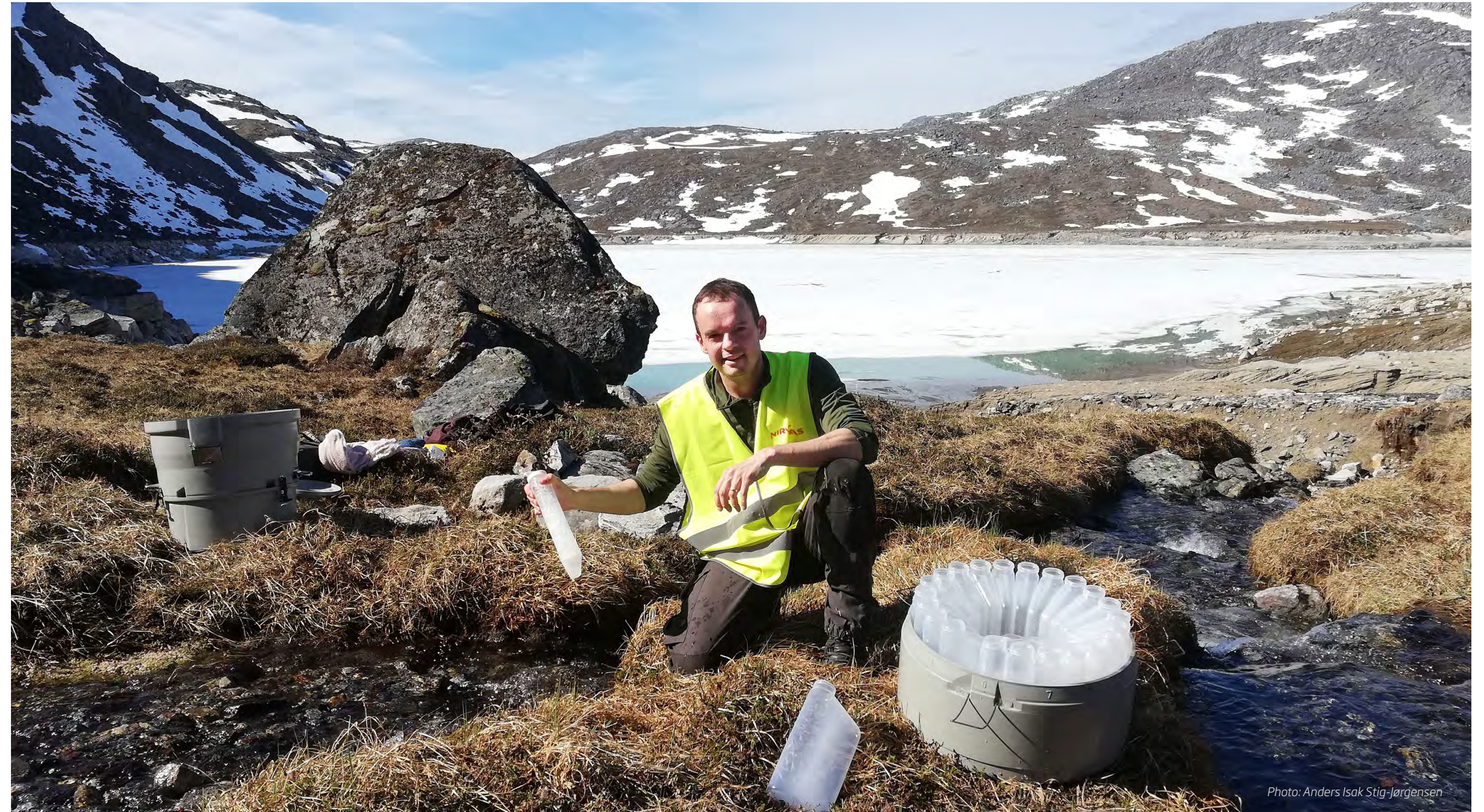
NIRAS Greenland has been conducting environmental monitoring for Greenland Ruby in southwestern Greenland since 2018. Anders Isak Stig-Jørgensen is seen here taking samples with an ISCO autosampler in a tributary to the project's tailings depot, which is located at the bottom of the lake in the background. The monitoring begins in early spring when ice and snow melt and ends in late autumn, when the environment freezes over again. NIRAS Greenland conducts environmental monitoring on several projects in Greenland.
